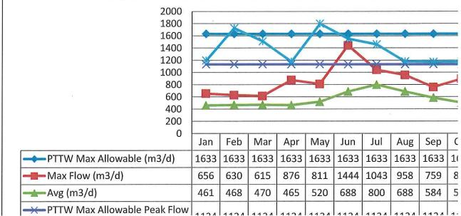
The above table shows there were exceedances in <u>instantaneous</u> peak flow rate (L/min) these occurrences were caused during pump start-up/pump to waste. The significant spike in May was due to scheduled Flow Meter calibration. The significant spike in June was due to a low pressure within the distribution system, which resulted in re-filling the water tower.
